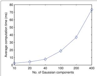
**Fig. 5** Average computation time of the proposed noise estimation with different Gaussian numbers at 10 dB SNR in white noise environment
