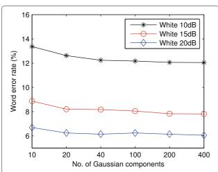
**Fig. 3** Word error rates of the proposed algorithm with different numbers of Gaussian components
