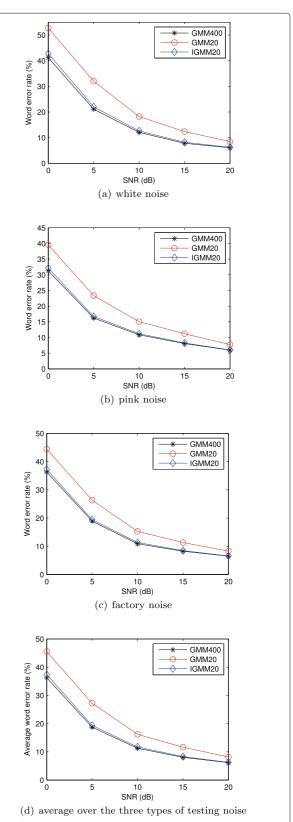
**Fig. 4** Performance comparison of the proposed algorithm (IGMM20) and original GMM-based feature compensation (GMM400 and GMM20) with different SNRs for the three types of testing noise
