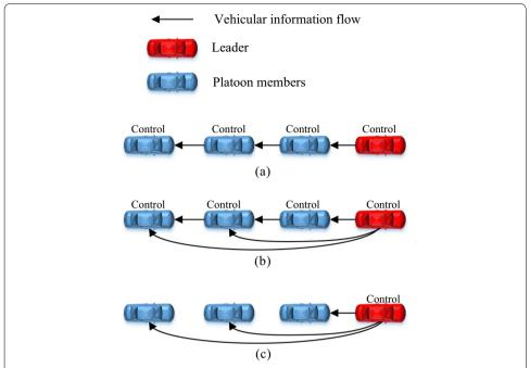
**Fig. 3** Typical platooning control schemes. **a** Decentralized control under PF. **b** Decentralized control under PLF. **c** Centralized control by leader
