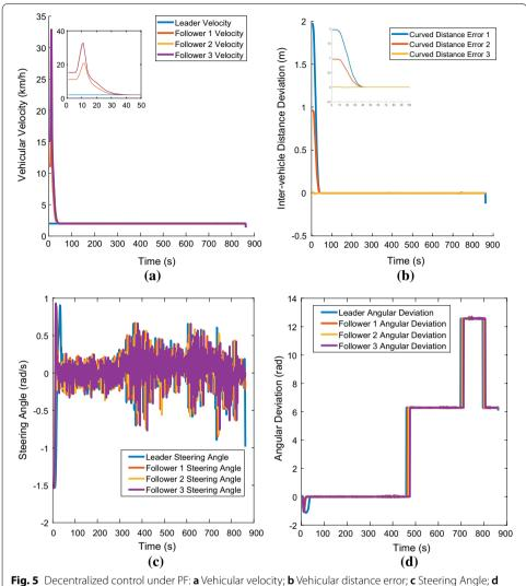
**Fig. 5** Decentralized control under PF: **a** Vehicular velocity; **b** Vehicular distance error; **c** Steering Angle; **d** Angular Deviation
