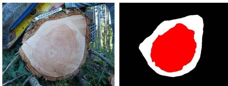
Fig. 16 Raw RGB image of log #1 from tree #1 taken in the forest (on the left) and the corresponding manually segmented image (on the right). On the segmented image: The white area is the sapwood located between heartwood and bark; the red area is the heartwood
