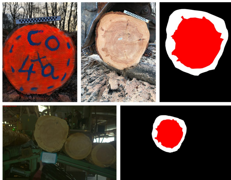
Fig. 5 Images of log C04a: Painted small end and large end images taken on the logyard, and corresponding manually segmented image (first row); large end image taken on the sawmill line and corresponding manually segmented image (second row). On the segmented images: The white area is the sapwood located between heartwood and bark; the red area is the heartwood
