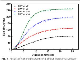
**Fig. 4** Results of nonlinear curve fitting of four representative leafy vegetables in MBPPSA model
