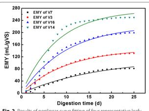
**Fig. 2** Results of nonlinear curve fitting of four representative leafy vegetables in first-order kinetic model
