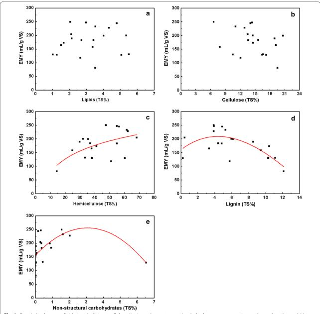
Fig. 1 Correlation between lipids, hemicellulose, cellulose, lignin, and non-structural carbohydrates contents and experimental methane yield (a-e, respectively) of 20 kinds of leafy vegetables
