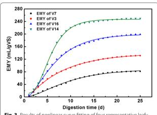
**Fig. 3** Results of nonlinear curve fitting of four representative leafy vegetables in modified Gompertz model
