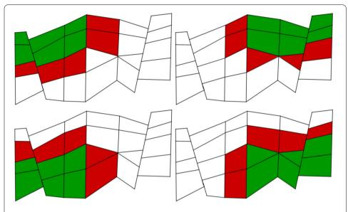
**Figure 2** An illustrative example of 4-way mesh partitioning. The interior cells of each of the four subdomains are colored green, while ghost cells are colored red
