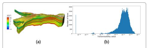
**Figure 3** Permeability distribution (**a**) in the x direction of the Norne grid. A histogram plot (**b**) of the transmissibility associated with cell interfaces from the Norne reservoir simulation case. The spike in the left end of the plot represents transmissibilities with value 0
