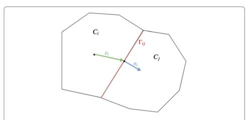
**Figure 1** A sketch of the geometric properties needed to calculate the static transmissibility (Eq. (9)) between two neighboring grid cells  $C_i$  and  $C_i$
