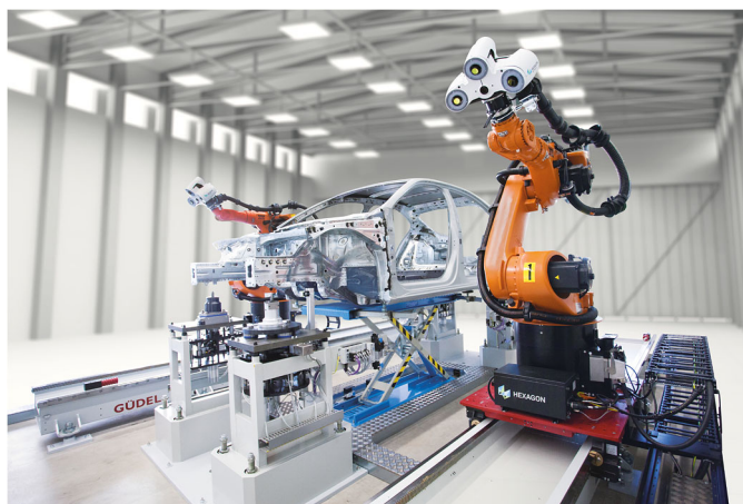
Figure 3 An exemplary setup of a 360° SIMS flexible measurement system. Image courtesy of Hexagon Manufacturing Intelligence.
