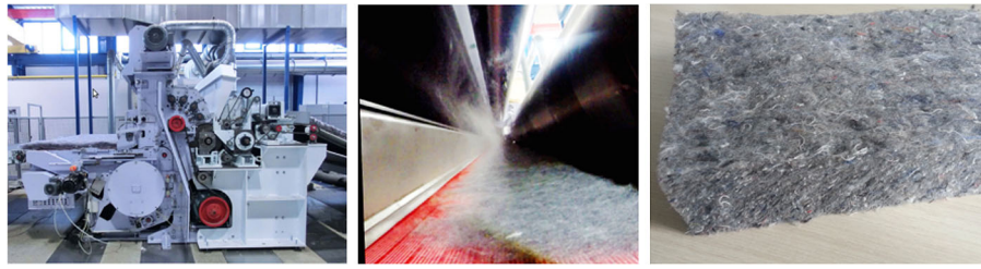
Figure 1 Industrial production of airlay fabrics. From left to right: Airlay machine (Airlay-K12 by machine manufacturer AUTEFA Solutions), aerodynamic web forming, nonwoven material.
