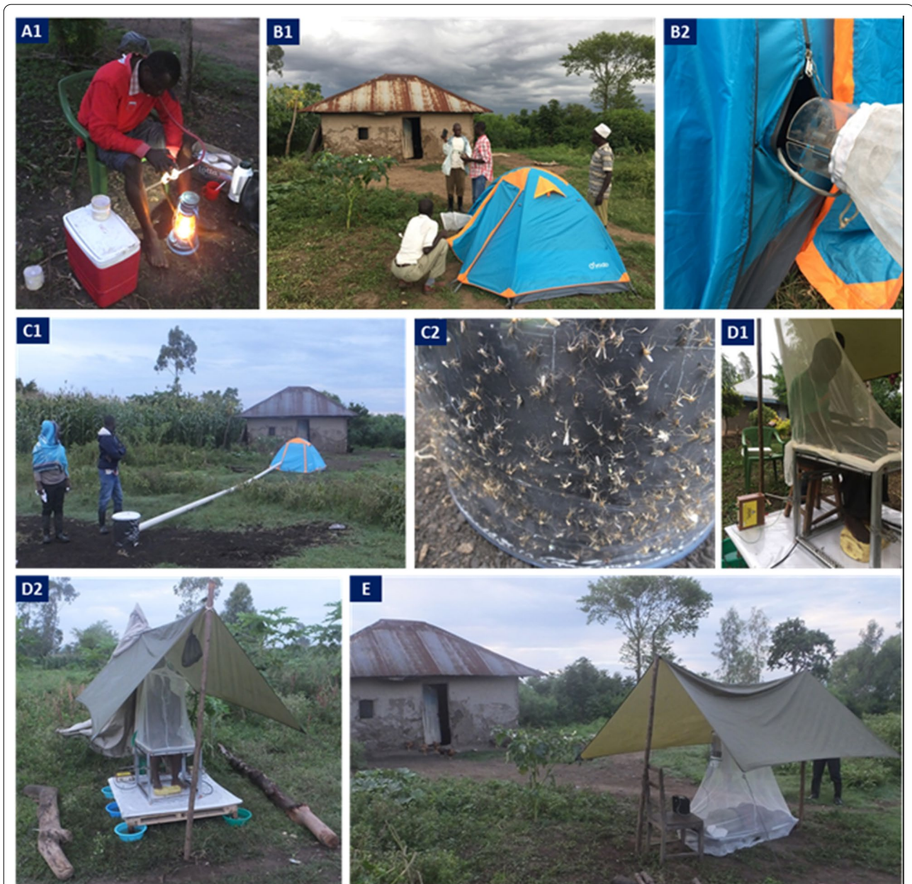
Fig. 2 Photographs showing the five outdoor trapping methods that were compared. A1 Human landing catch (HLC), B1 Furvela tent trap (FTT), B2 FTT opening with CDC light trap (light removed) attached, C1 human decoy trap (HDT), showing tube taking human odour to the heated cylinder sticky trap, C2 HDT, showing mosquitoes stuck to sticky panel on heated cylinder, D1, 2 electrocuting grid trap (EGT), E outdoor CDC light trap (CDC LT), hung next to human sleeping inside an untreated bed net
