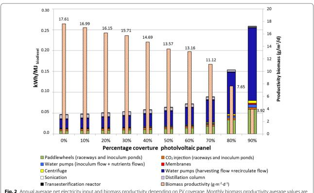
Fig. 2 Annual average net electricity input and biomass productivity depending on PV coverage. Monthly biomass productivity average values are indicated above bars
