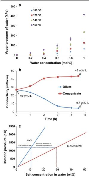
**Fig. 2** Challenges related to high IL dehydration in current IL separation methods: **a** distillation, **b** electrodialysis and **c** reverse osmosis. Detailed information on Fig. 2b is described in Additional file 1: Figure 57; data in Fig. 2c on upper limit of osmotic pressure for an industrial setting were obtained from Reference [20]
