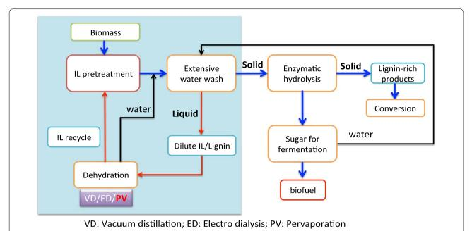
**Fig. 1** Simplified process flow diagram for the potential ionic liquid-based biorefinery and performance evaluation of pervaporation, ED and VD in one of the water-wash process scenarios
