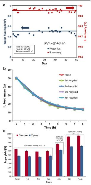
Fig. 6 Stability of the pervaporation membrane as a function of time and usage (a and b), and performance of recycled IL for biomass pretreatment (c). Biomass loading in pretreatment step is fixed at 10 wt%
