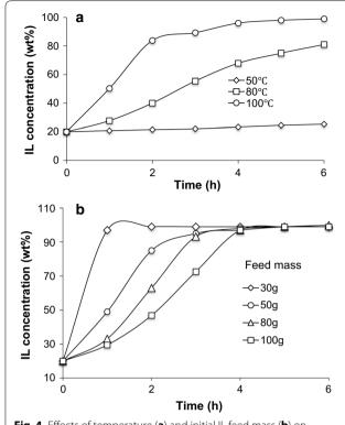
**Fig. 4** Effects of temperature (**a**) and initial IL feed mass (**b**) on  $[C_2C_1\text{Im}][OAc]$  concentration as a function of time (@ 100 °C)
