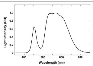
**Fig. 8** Spectral properties of LED light source used for *C. gracilis* culture. Wavelength-dependent intensity determined using a spectrometer BRC115 (B&W Tek, Inc., Newark, DE, USA) and normalized at peak wavelength
