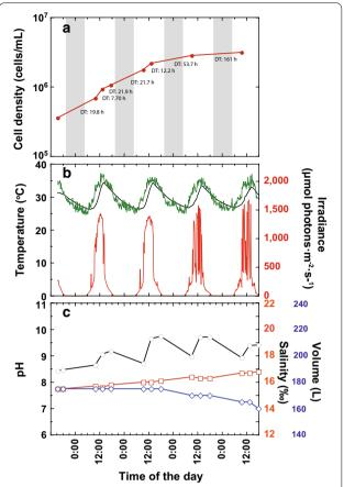
**Fig. 7** Open-air large-scale cultivation of *C. gracilis.* **a** Changes in cell density. DT designates doubling time between two consecutive time points. **b** Changes in ambient air, water temperatures, and irradiance (*green, black,* and *red lines,* respectively). **c** Changes in pH, salinity, and volume of culture medium (*black, red* and *blue lines,* respectively). Experiment performed from August 3 to 7, 2015
