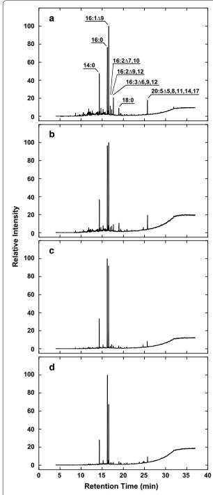
**Fig. 3** GC–MS chromatograms of FAME derived from *C. gracilis* cells grown in F/2-enriched seawater without vitamins. Cells harvested at day 2, 4, 7, and 10 (**a–d**, respectively) after culture start; extracted lipids methyl-esterified and subjected to GC–MS; and peak identities indicated on **a**
