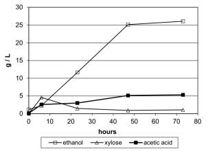
**Fig. 4** Fermentation of detoxified hemicellulose extract. Strain M1732 was grown in TSC7 medium containing hemicellulose extract at 1 L volume at 51 °C at pH 5.8. The fermentor contained 42 g/L available sugar (76 % xylose, 11 % mannose, 6 % glucose, 5 % galactose, and 2 % arabinose, as polymeric hemicellulose) at the start, and was fed an additional 25 g/L over two feedings at 24 and 47 h. The hemicellulose was detoxified by lime treatment and nanodiafiltration
