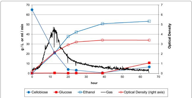
**Fig. 1** Fermentation of cellobiose and maltodextrin. Strain M1151 was grown in TSC3 medium containing 90 g/L maltodextrin and 60 g/L cellobiose at 1 L scale. Cellobiose, glucose, and ethanol levels are shown in units of g/L on the *left axis*
