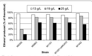
**Fig. 3** Strain comparison in varying levels of hemicellulose extract. *Bars* indicate ethanol produced in batch fermentations as a percent of the maximum theoretical ethanol possible for the amount of sugar provided by the extract, indicated by *bars*: 13 g/L (*white*), 19 g/L (*gray*), and 25 g/L (*black*)
