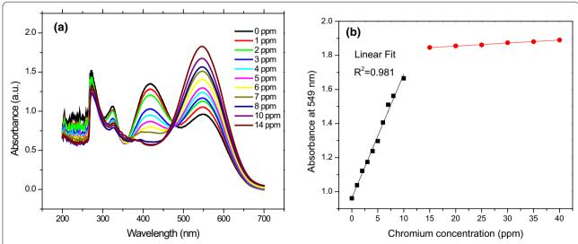
Fig. 3 a Plot of change in the UV–visible spectra of **compound 4a** at different concentrations of chromium ions; **b** the linear relationship between chromium concentration and absorbance intensity
