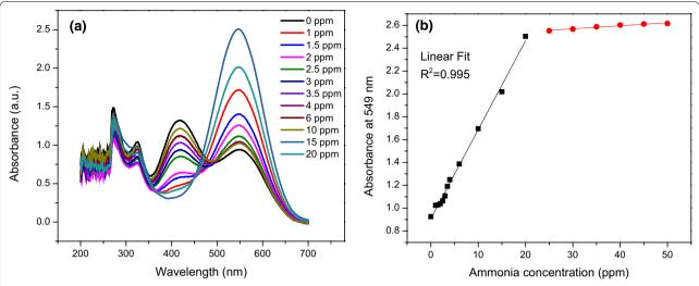
**Fig. 2** a The plot of changes in UV–visible spectra of **compound 4a** solution as a function of different ammonia concentrations (0–20 ppm), **b** the linear relationship between different ammonia concentrations and absorbance intensity at 549 nm wavelength
