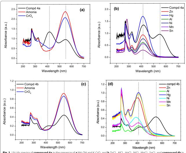
**Fig. 1** UV–Vis spectra of **compound 4a** in the presence of **a** NH<sub>4</sub>OH and K<sub>2</sub>CrO<sub>4</sub> and **b** ZnCl<sub>2</sub>, AlCl<sub>3</sub>, HgCl<sub>2</sub>, NiCl<sub>2</sub>, MnCl<sub>2</sub>, SnCl<sub>2</sub> and **compound 4b** in the presence of **c** NH<sub>4</sub>OH and K<sub>2</sub>CrO<sub>4</sub> and **d** ZnCl<sub>3</sub>, AlCl<sub>3</sub>, HgCl<sub>2</sub>, NiCl<sub>2</sub>, SnCl<sub>2</sub>
