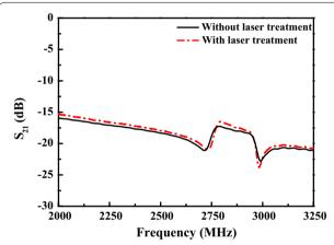
**Fig. 7** Resonant frequency of SMR filters with as-deposited and annealed AIN films
