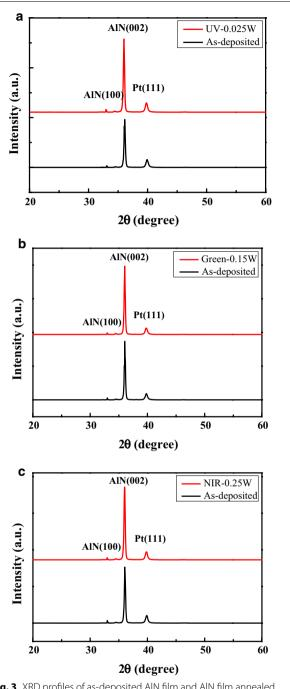
**Fig. 3** XRD profiles of as-deposited AIN film and AIN film annealed using three laser systems: **a** UV, **b** green and **c** NIR
