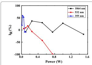
**Fig. 4** Relative improvement in (002) peak intensity as function of laser power for laser systems with different wavelengths
