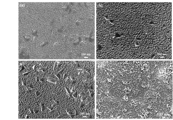
Fig. 5 SEM images of as-deposited and UV-annealed AIN films: a as-deposited, b 0.025 W, c 0.05 W and d 0.1 W
