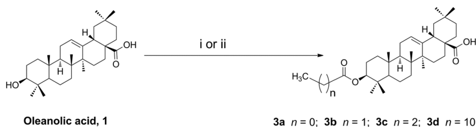
Scheme 1 Synthesis of acyl oleanolic acid derivatives. Reagents and conditions: (i) anhydride, DMAP, anhydrous \text{CH}_2\text{Cl}_2 /pyridine, rt (64–89%); (ii) acyl chloride, \text{Et}_3\text{N} , anhydrous THF, rt (75–88%)
