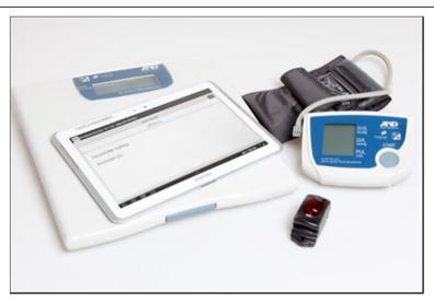
Fig. 1 The telehealth system, Telekit, consists of a tablet, a fingertip pulse oximeter, a blood pressure monitor, and a scale
