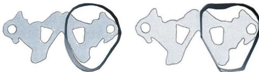
Fig. 7 Illustration of geometry modifications. The CAT-CAM socket on the left follows widely the limb anatomy; the MAS socket on the right is more aggressive in defining the limb shape (adapted from Psonak, Richard. "Transfemoral prostheses" in orthotics and prosthetics in rehabilitation , Oxford, Elsevier, 2 nd Edition, 2007: 652-684)
