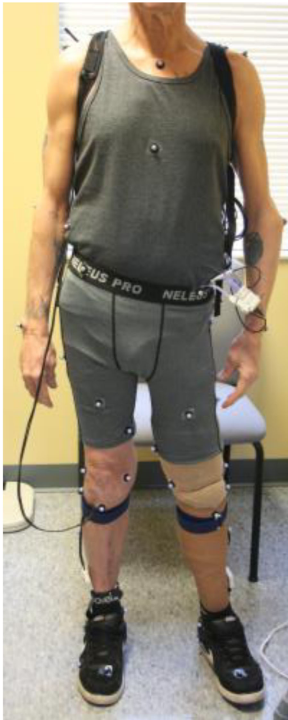
Fig. 11 Reflective markers on a transfemoral amputee. Conventional motion capture will be used to measure overall body motion during gait
