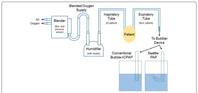
Fig. 1 Schematic showing the primary components of a bubble nCPAP circuit. The differences in conventional and Seattle-PAP bubbler devices are shown. All other elements of the CPAP circuit are identical between the groups
