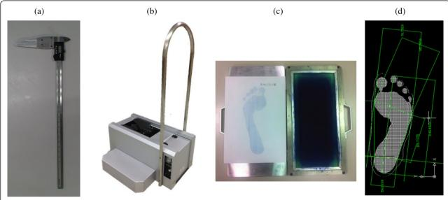
Figure 1 The four measurement methods: digital caliper (a), 3D foot scanner (b), Harris mat (c) and digital footprint image (d).
