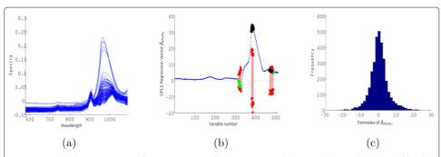
**Fig. 4** (a) Overall 110 NIR spectra for temperatures of 30, 40, 50, 60, and 70 °C are shown. Illustration of (b) the regression vector  $\hat{\beta}_{OPLSb_i}$  and (c) the empirical null distribution of the realized  $\hat{\beta}_{OPLSb_i}$  are shown for the NIR spectra. The wavelength ranges of the selected variables were from 960 to 970 nm ( $x_{381}$  to  $x_{391}$ ) and from 1049 to 1060 nm ( $x_{470}$  to  $x_{481}$ )
