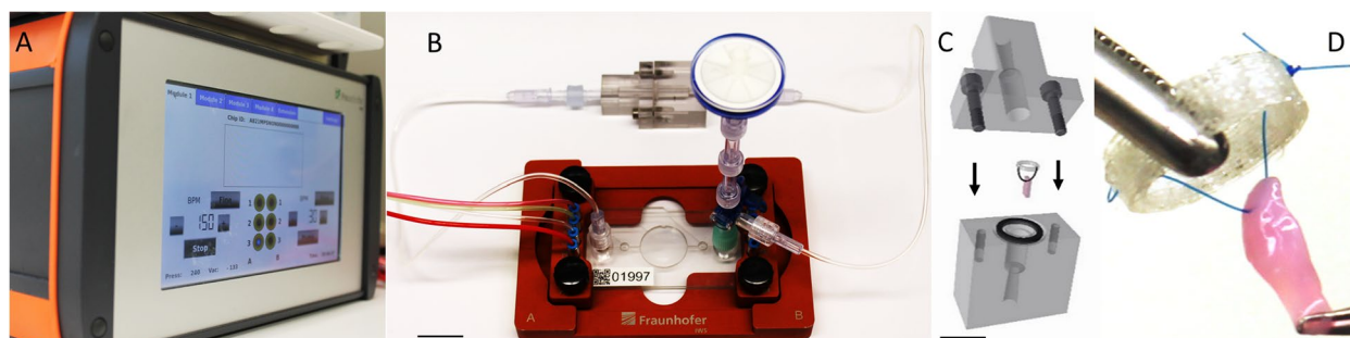
Fig. 3 MPS-TIC Setup: A The MPS control unit enables regulation of pumping sequence and pneumatic pressure; B The high flow setup is conjoined with the attenuation element (here shown without culture medium); C The AV tissue specimen is stitched to a TPU ring and inserted into the tissue incubation chamber (TIC) (Arrows: flow direction [Q], scale bar: 1 cm). D Example of a stitched (TPU ring) pAV specimen prior insertion in the TIC
