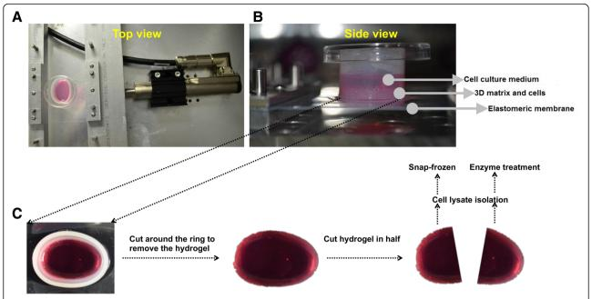
**Fig. 1** Schematic diagram showing the **a** top and **b** side views of the cyclic stretch culture bioreactor used in this study. **c** Schematic of the methods to collect cell lysate for phosphorylated and total protein analysis in this study
