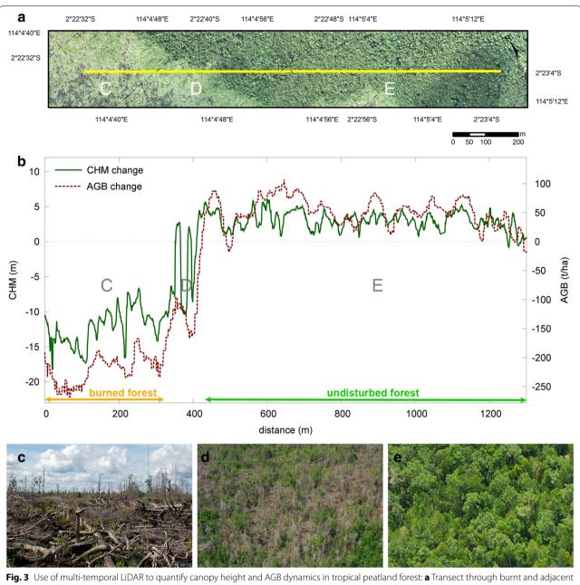
Fig. 3 Use of multi-temporal LiDAR to quantify canopy height and AGB dynamics in tropical peatland forest: **a** Transect through burnt and adjacent undisturbed peat swamp forest. **b** Changes in canopy height and AGB associated with different forest conditions; and photographs of **c** burnt forest, **d** transition area and **e** undisturbed forest (Courtesy of [16])
