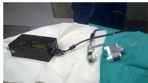
Fig. 1 Vibration transmittance measurement device. Main unit, actuator and sensor (from left to right)
