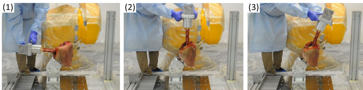
Fig. 8 Documentation of manual flexion–extension of the human hip joint: images (1), (2), (3) present three selected positions from the movement
