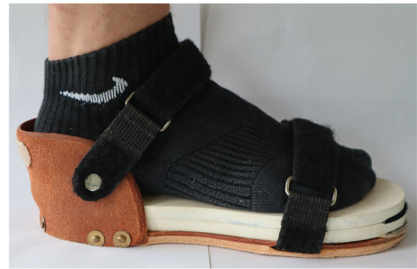
Fig. 2 Custom-built sandal with added insoles to simulate LLI. The sandal was available in three different sizes to accommodate the subjects
