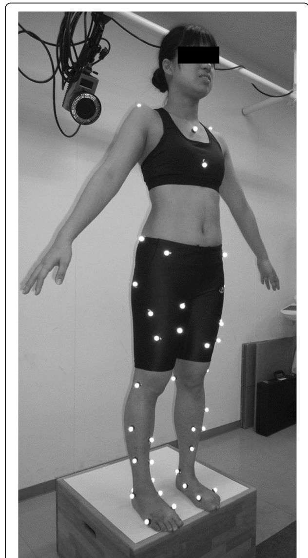
Fig. 2 Marker locations. A total of 46 retro-reflective markers (14 mm in diameter) were placed at standard anatomical landmarks
