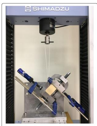
Fig. 2 Experimental setup of the biomechanical testing
