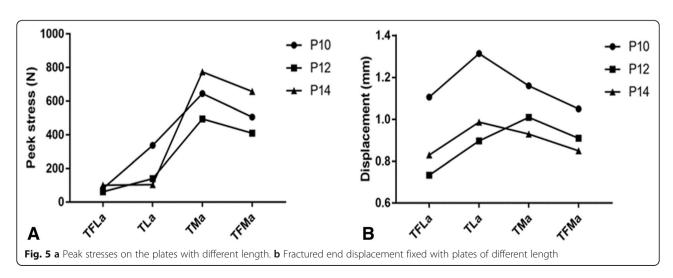
of the tibia, the displacement in models fixed with P10 was the highest while that in models fixed with P12 showed the smallest value. In models with plates implanted on the medial side of the tibia, the displacement in models fixed with P10 was the highest as well while that in models fixed with P14 showed the smallest value.
