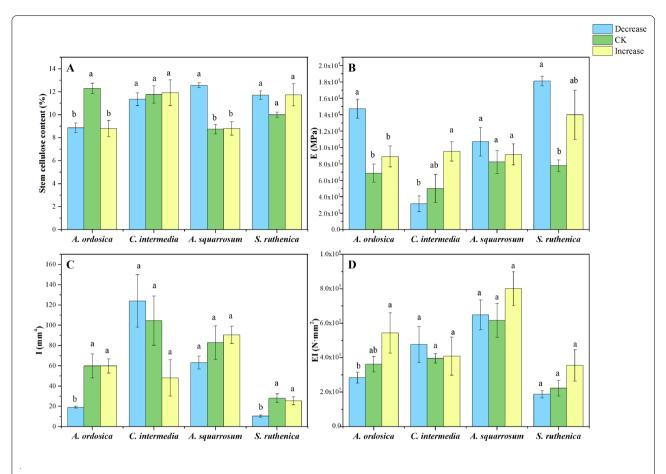
Fig. 5 Shoot property traits linked to wind resistance in four plant species under different wind treatments: a Stem cellulose content, b Young's modulus (E), c Second moment of area (I), and d Flexural stiffness (EI). Decrease, CK (ambient) and Increase refer to wind velocity treatments. Different lowercase letters indicate significant differences among treatments at p < 0.05. The error bars are plotted by means  $\pm$  SE
