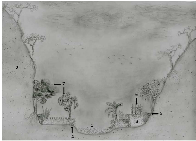
Fig. 3 Profile of the river basin section and the location of tajos describing tajos. 1) River, 2) mountain slope, 3) lamedal , 4) tajos stone-walls, 5) acequias , 6) crops, 7) perennial vegetation
