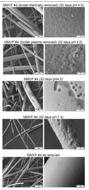
**Fig. 4** MMVF #4 (high-alumina) morphology by various dissolution conditions at pH 4.5 and pH 7.4, with and without binder: SEM analysis
