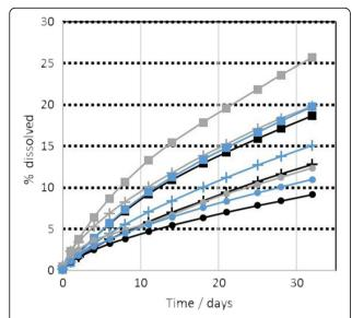
**Fig. 5** Binder effects on dissolution kinetics at pH 4.5 of MMVF #4, with binder (*dots*), binder removed by plasma (*crosses*), binder removed thermally (*boxes*) for the three oxides Si (*black*), Al (*blue*), Mg (*grey*)
