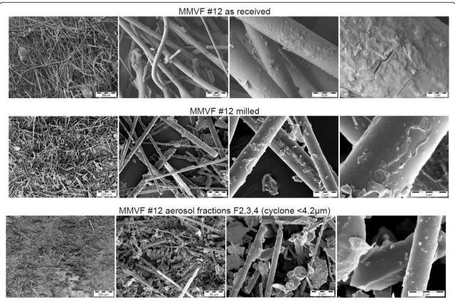
Fig. 1 SEM micrographs of MMVF #12. As received – after milling – only respirable fraction. See the Supporting Information for analogous results on MMVF #5
