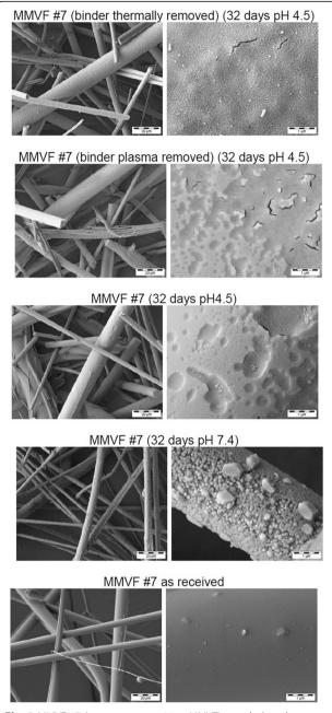
**Fig. 3** MMVF #7 (average composition MMVF) morphology by various dissolution conditions at pH 4.5 and pH 7.4, with and without binder: SEM analysis
