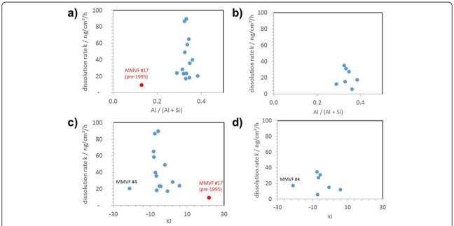
**Fig. 6** Summary of measured dissolution rates k [Si,Al, ng/cm²/h] as a function of the compositional parameters **a,b** of the molar ratio Al / (Al + Si) or **c,d** of Kl. The flow rates are identical throughout, and the pH is **a,c** pH 4.5 and **b,d** pH 7.4. The materials with highest k at pH 4.5 (MMVF #1, MMVF #5) were also screened at pH 7.4 and are included in the plot
