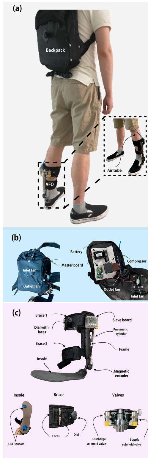
Fig. 1 System overview (a) Picture of a person wearing an ankle-foot orthosis (AFO) with a backpack. (b) The backpack, as a pneumatic power source, comprises a compressor, battery, master board, and both inlet/outlet fans for heat dissipation. (c) The AFO consists of a pneumatic actuator, frame for fixation, and an insole. An air tube is connected between the compressor and pneumatic cylinder. Two ground reaction force (GRF) sensors are located on the toe and heel for gait phase detection. Calf braces placed in the top and the middle of the frame connect the AFO with the human leg and contribute to the high force transmissibility via a stable fixation of the static part of the pneumatic cylinder to the calf. The dial, including the laces in the brace, enables the adjustment of the fixation of the AFO frame to the calf. Supply and discharge solenoid valves are implemented for AFO control based on the GRF sensor signal
