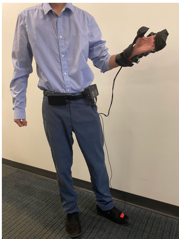
Fig. 6 Illustration of the NuroSleeve system in operation. The MCU and battery are worn on the belt, while an IMU sensor attached to the shoe controls the splint motor in continuous mode
