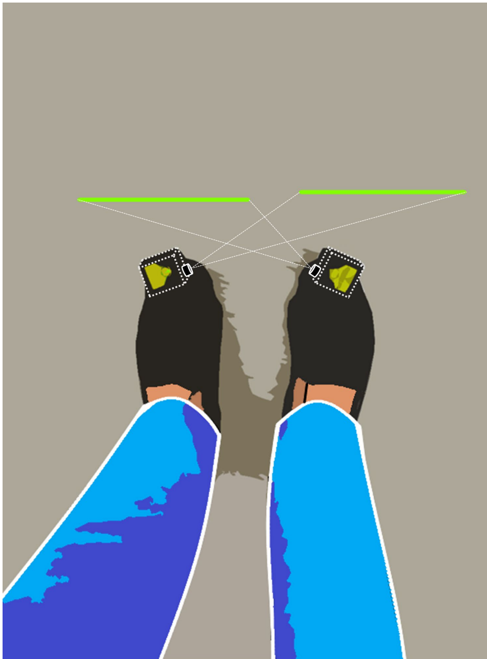
Fig. 1 Illustration of the experimental setup for the visual cueing with laser-beam
