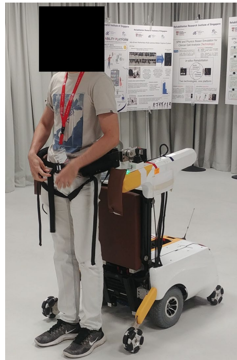
Fig. 1 Mobile Robotic Balance Assistant (MRBA) with a user attached to it
