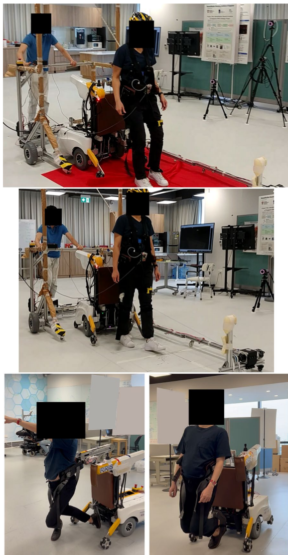
Fig. 12 Top: An FE_SL trial that involved FIMP to trigger slip by pulling the subject’s left ankle forward when the left foot struck the sliding sheets. Middle: An FE_KB trial that involved FIMP to trigger knee buckling by pulling the subject’s left knee forward during left mid-stance. Bottom left: An FS_RO trial in which the subject fell when reaching out to grab an object. Bottom right: An FS_W trial in which the subject fell when walking
