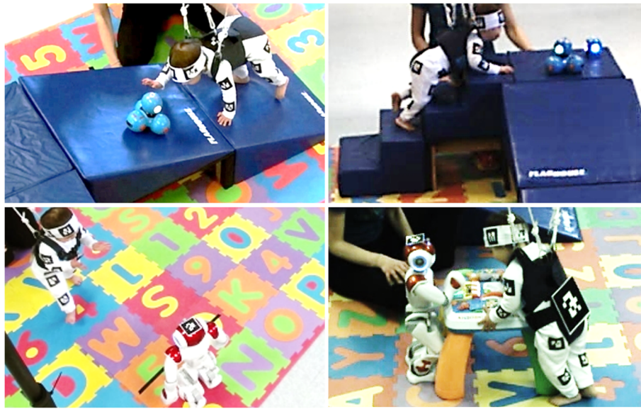
Fig. 6 Snapshots of a child within the GEAR system. The child, supported by the device, performs various and complex motor actions and interacts with the robots during exploration and manipulation of the objects of the enriched environment
