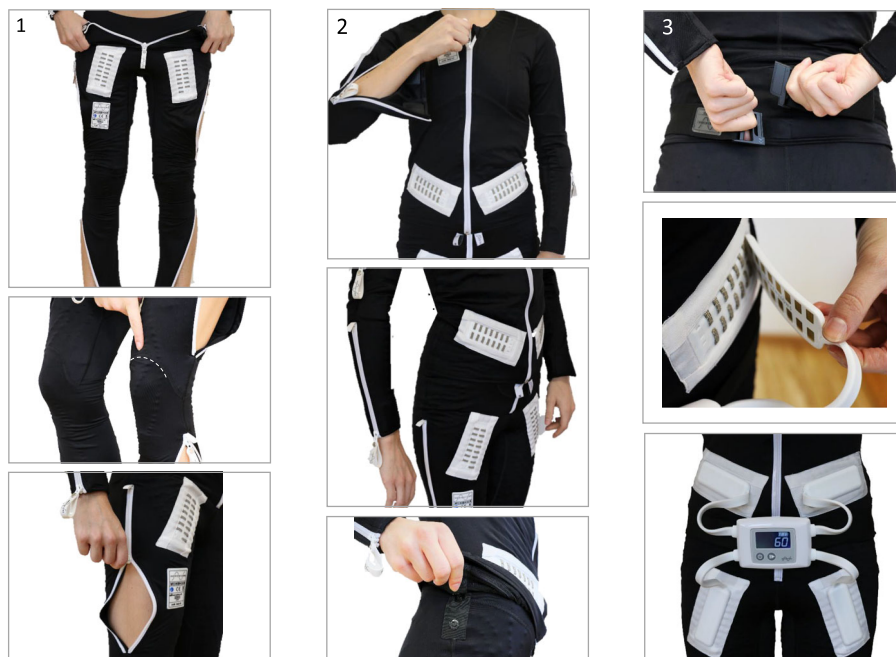
Fig. 1 Donning of the Mollii® suit – trousers [1] and jacket [2] and connection of the control unit to the suit [3]
