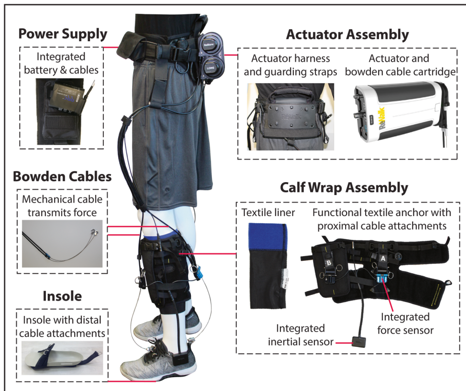
Fig. 1 The ReWalk ReStore™ consists of an actuator assembly, calf wrap assembly, and shoe insole. A power supply is integrated into the actuator assembly. Bowden cables span these components to transmit assistive forces generated by the actuator to the ankle. More specifically, two Bowden cables are used in the ReStore™, each having attachment points proximal (on the Calf Wrap Assembly) and distal (on the Insole) to the ankle. One of the cables is located anterior to the ankle and the other is located posterior to the ankle. When the anterior cable is retracted, an ankle dorsiflexion torque is produced. When the posterior cable is retracted, an ankle plantarflexion torque is produced
