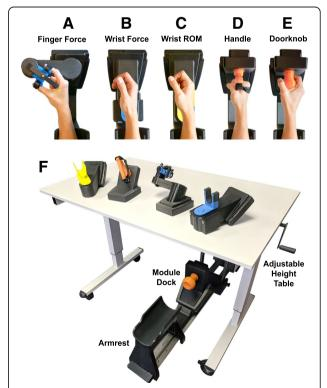
**Fig. 1** Suite of hand and wrist assessment devices. Images of the finger flexion/extension device (**a**), the wrist flexion/extension devices (**b/c**), the wrist rotation device with the D-grip handle (**d**) and with the doorknob manipulandum (**e**), and the testing table used for assessing cSCI participants (**f**)
