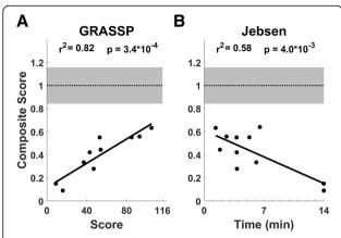
**Fig. 7** Motor function measured using the devices is correlated with standard assessments. Normalized composite score integrating performance on all devices is highly correlated with total GRASSP score (a) and moderately correlated with score on the Jebsen Hand Function Test (b). The grey areas indicate SD of the control group's composite scores
