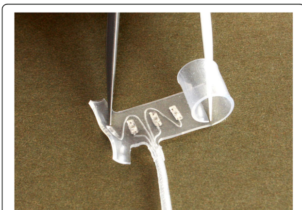
Fig. 1 Standard spiral nerve cuff electrode. Caption: A standard self-sizing spiral nerve cuff electrode ( d = 4 mm) licensed from Case Western Reserve University. In this study, 14 human participants were implanted with spiral cuffs on ten different nerves. Photo courtesy of Ardiem Medical, Inc. [48]
