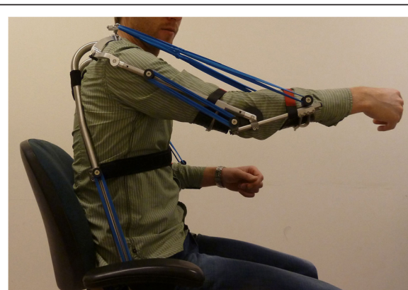
Fig. 1 The prototype arm support worn by a healthy user
