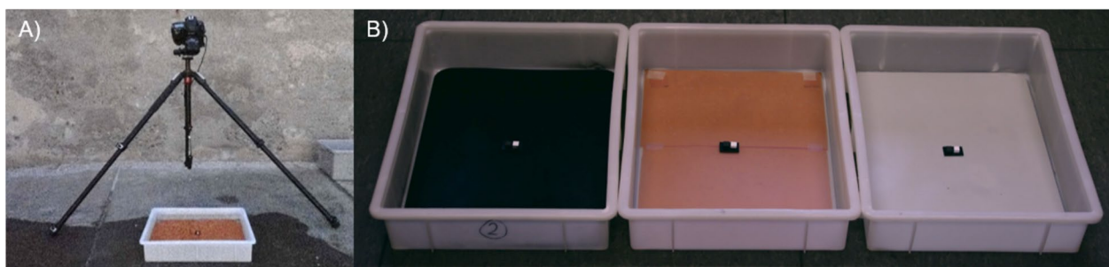
Fig. 6 Setup of experiment 1. A Overview of the setup, B trays with the three backgrounds used in the first experiment (from left to right: dark/grey , medium/orange , light/grey )
