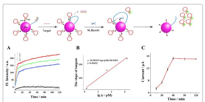
**Fig. 4** A Fluorescence kinetics curves of the nanomachine with addition of 10 U Nt.BsmAl and target BCR/ABL fusion gene at different concentrations (from a to d:  $2 \mu M$ , 2 n M, 2 p M and blank, separately). **B** The relationship between the slope of tangent at t = 0 s and logarithmic value of target BCR/ABL fusion gene concentrations (range of concentration: 2 p M, 2 n M, and 2 u M separately). **C** Time optimization of intermediate DNAs hybridizing with the capture DNA
