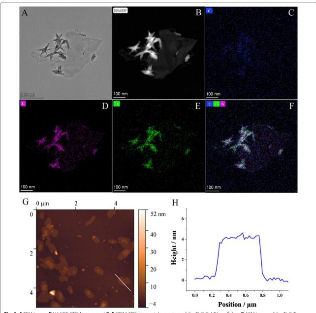
**Fig. 1** A TEM image, **B** HAADF-STEM image and **C**–**F** STEM-EDS elemental mappings of the  $Ti_3C_2T_x$  MXene flakes. **G** AFM image of the  $Ti_3C_2T_x$  MXene flakes and **H** the height profile along the white line
