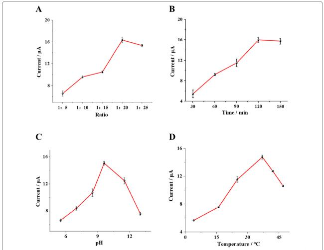
Fig. 5 Optimization of experimental conditions: A ratio of walker to support DNA, B cleaving time of Nt.BsmAl nicking endonuclease, C pH of DEA buffer, D cleaving temperature of Nt.BsmAl nicking endonuclease. The error bars represent the standard deviation of three parallel measurements
