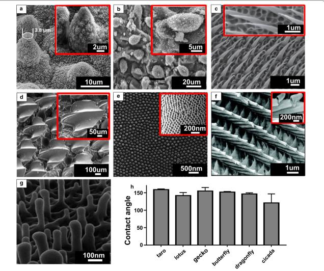
Fig. 1 SEM images of nano-structured surfaces of: **a** lotus leaf [20, 146], **b** taro leaf [56], **c** gecko skin [147], **d** shark skin [148], **e** cicada wing [149], **f** butterfly wing [150] and **g** dragonfly wing [18]; **h** contact angles of naturally occurring bactericidal surfaces. Figures reproduced with permission
