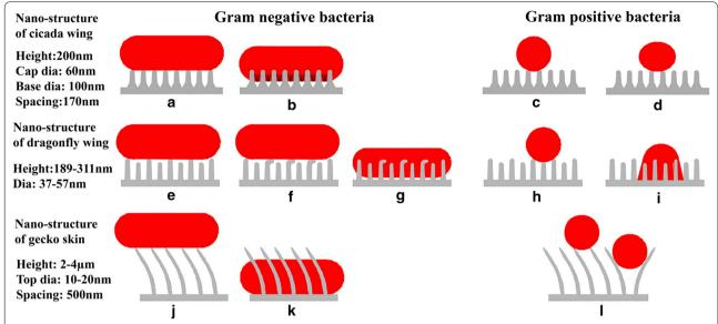
**Fig. 4** Schematic showing bacteria-nano-structured surface interaction of: **a, b** cicada wing and gram-negative bacteria, **c, d** cicada wing and gram-positive bacteria, **e-g** dragonfly wing and gram-negative bacteria, **h, i** dragonfly wing and gram-positive bacteria, **j, k** gecko skin and gram-negative bacteria and **i** gecko skin and gram-positive bacteria. Nano-structure dimensions are indicated next to each species, dimensions not to scale
