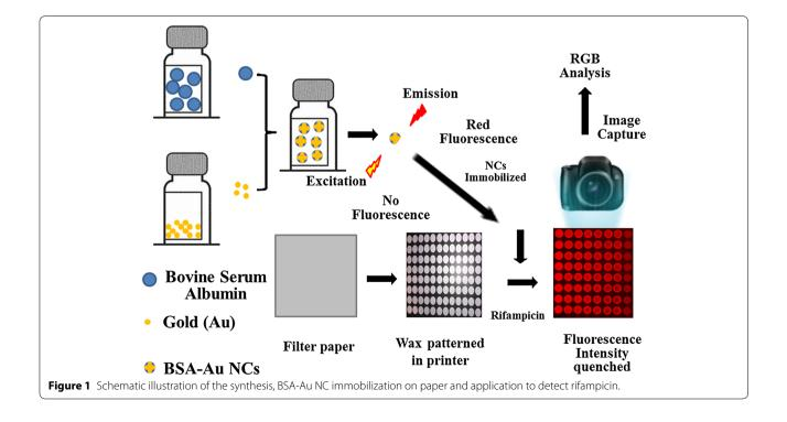
melting wax to form hydrophobic barriers, and immobilizing the BSA-Au NCs in the reaction zones. After dropping the samples onto the paper sensor, the fluorescence images are captured by a digital camera and analyzed [38–40].
