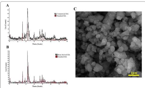
**Fig. 1** Evaluation of the purity of the extracted hydroxyapatite (HA); **A** commercial HA XRD spectrum, **B** XRD spectrum of extracted HA, XRD spectra showed that most of the mineral content was HA, **C** SEM images of the HA particles. The particle size of the extracted powder was estimated to be  $409.78 \pm 89.58$  nm
