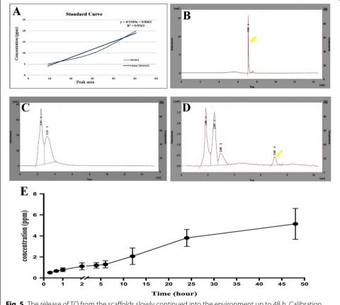
**Fig. 5** The release of TQ from the scaffolds slowly continued into the environment up to 48 h. Calibration curve for standard TQ (**A**), HPLC peak for a representative standard TQ (**B**), a representative sample in 60 s (**C**), and 24 h (**D**). The releasing curve of TQ from scaffold during 48 h (**E**)
