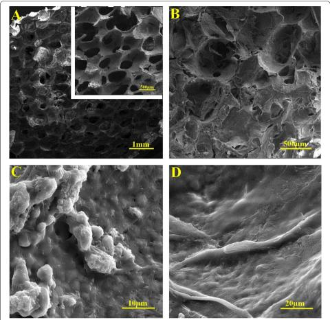
**Fig. 11** Scanning electron microscope images: **A** hydroxyapatite (HA) scaffold, **B** HA scaffold containing alginate, **C** osteoblastic cells with short processes in the 3D+TQ+OM group, **D** cells with mesenchymal stem cell phenotype expanded on 3D-TQ-OM cultures
