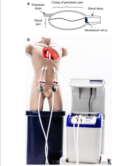
**Fig. 1** The newly developed RELIGA-EXT prosthesis (construction diagram and the complete heart support system)
