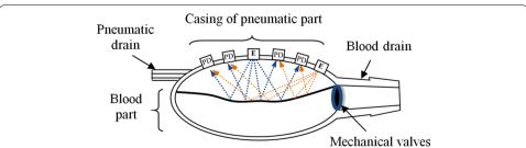
**Fig. 2** The idea of an optical measurement system with photodiodes (PD) and light emitting diode (E) in the pneumatic part casing
