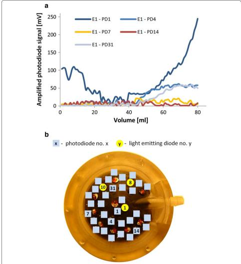
**Fig. 3** Relation between the actual volume and signals from each of the 32 photodiodes (**a**), when only light emitting diode E1 is used (**b**)
