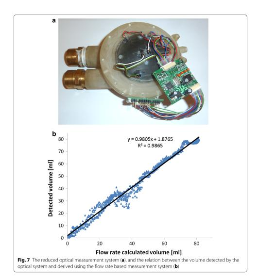
Knowing the required number of configurations, the size of the measurement system was reduced; the electronic circuit was redesigned to a more compact one. In order to reduce the size of the electronic circuit, a 4-layer transducer board was used. In Fig. 7a the reduced preliminary system is shown. Finally, the optical system was reduced to two light emitting diodes (E1, E8) and three photodiodes (PD1, PD15, PD32) marked in Fig. 6a.
