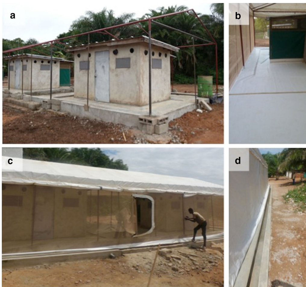
Fig. 3 Semi-field enclosure for release-recapture studies. a Metallic framework of the enclosure built around 2 experimental huts; b white tarpaulin floor to facilitate collection of dead mosquitoes; c netting walls and door, and tarpaulin roof; d water gutter to reduce entry of ants
