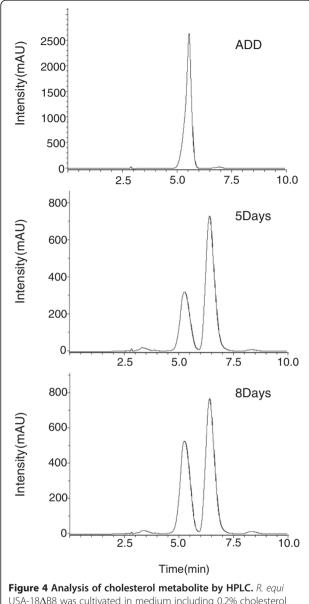
**Figure 4** Analysis of cholesterol metabolite by HPLC. *R. equi* USA-18ΔB8 was cultivated in medium including 0.2% cholesterol and 0.2% Tween 20 at 37°C, 200 rpm. The broth, harvested at the indicated time, was extracted with ethyl acetate and the compounds within were analyzed by HPLC using a reverse-phase column as described in Materials and methods.
