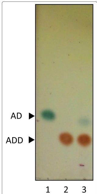
**Figure 6 Biotransformation of AD into ADD.** *R. equi* USA-18 $\Delta$ B8 was cultivated in glycerol minimal medium supplemented with 0.5% (w/v) AD and 0.2% (v/v) Tween 20 at 37°C, 200 rpm, for 5 days. The broth was extracted with ethyl acetate and the dissolved compounds were analyzed by TLC. Lane 1 and 2 are AD and ADD standards, respectively. Lane 3 is the ethyl acetate extract.
